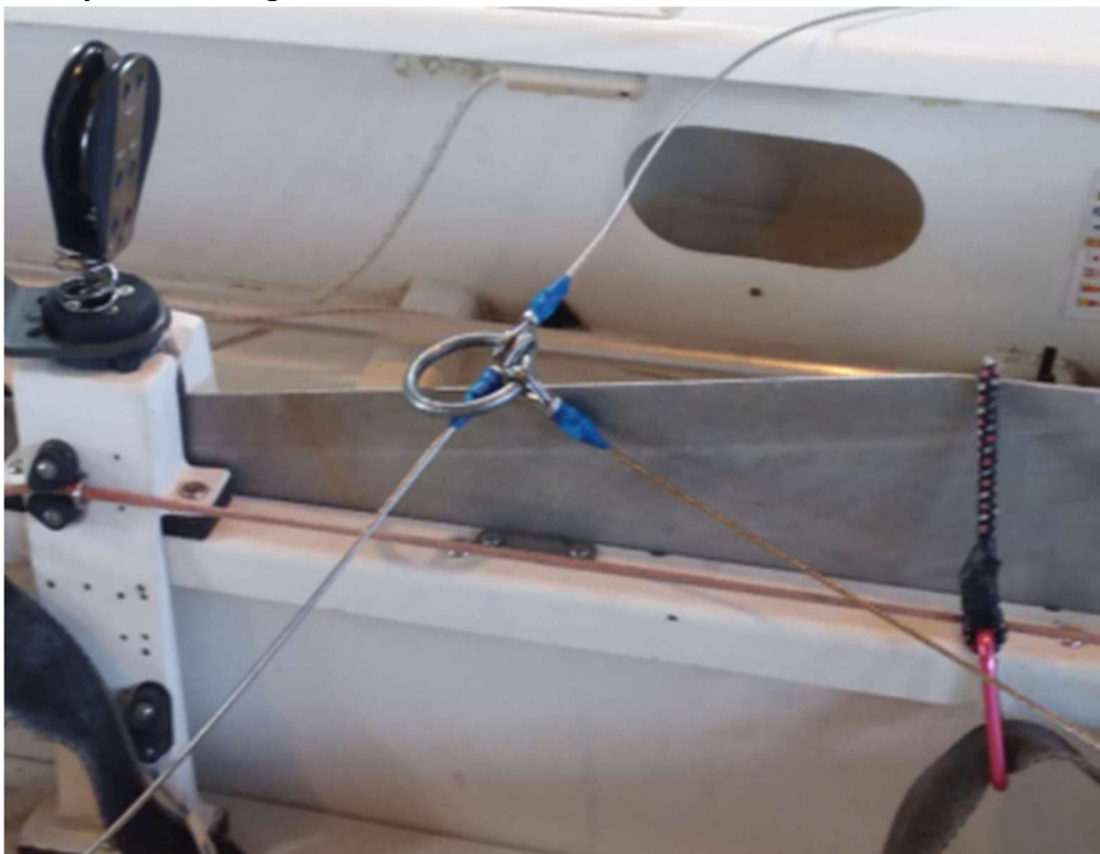
Newly made lifting bridle finished and tested:
