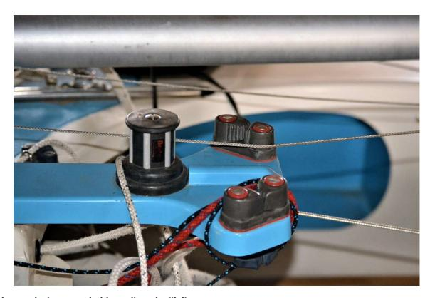
Winch to make it easy to hold or adjust the jib lines.
