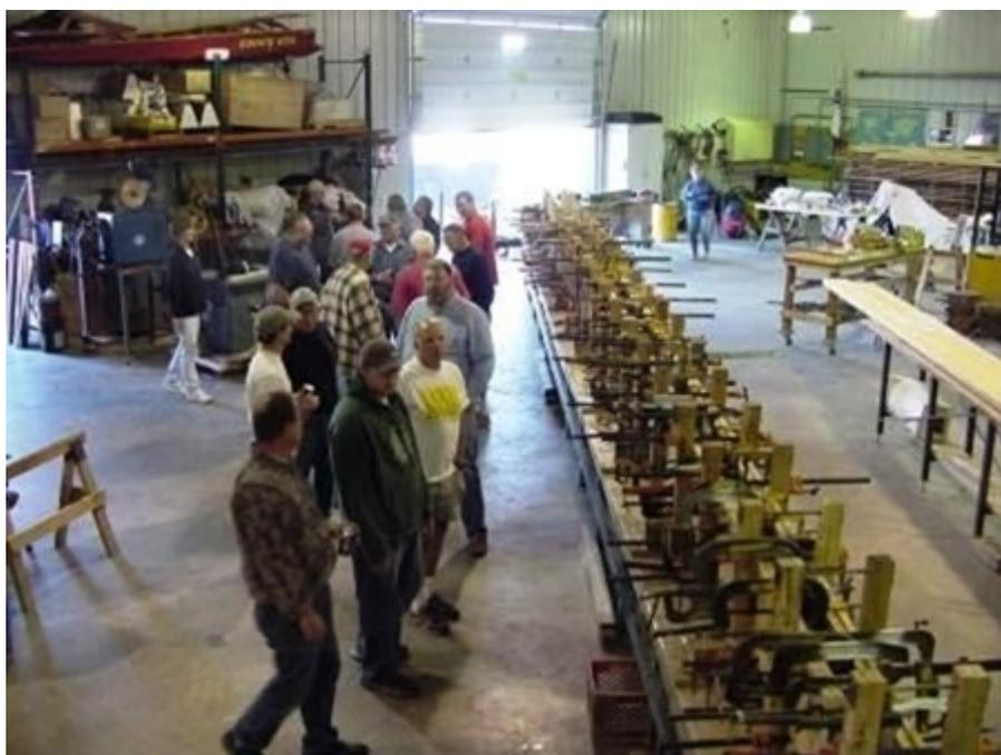
501 clamps were used to clamp up the Deuce backbone
