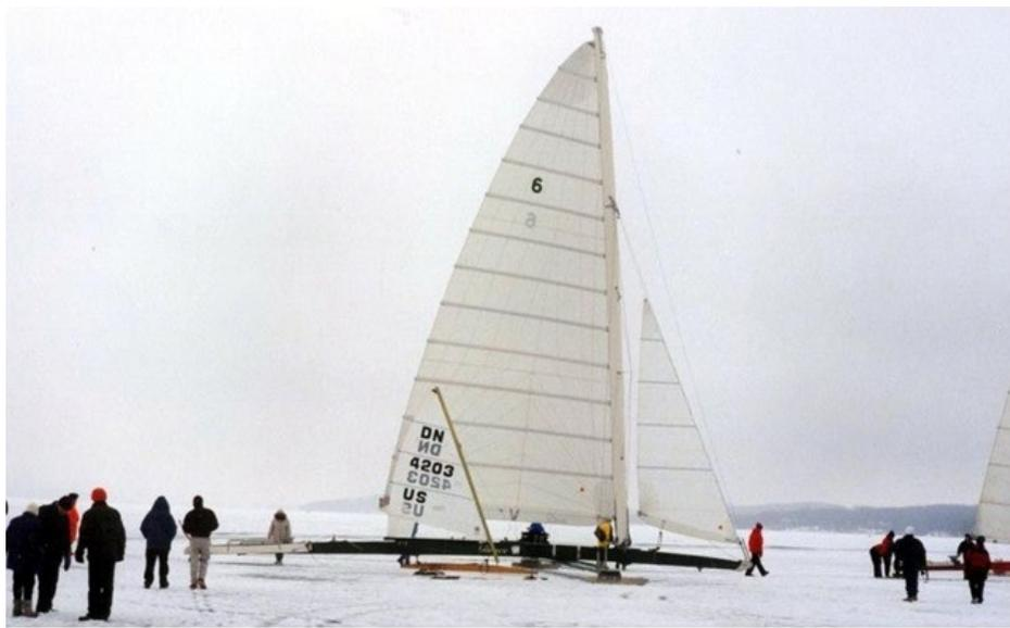
The Deuce, alongside a DN. The DN is 12 ft long with a 16 ft. mast. The Deuce is slightly larger
