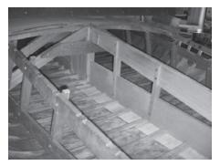
Shows the completed backbone structure and A-frame mast support. The A-frames were sound and reused.
