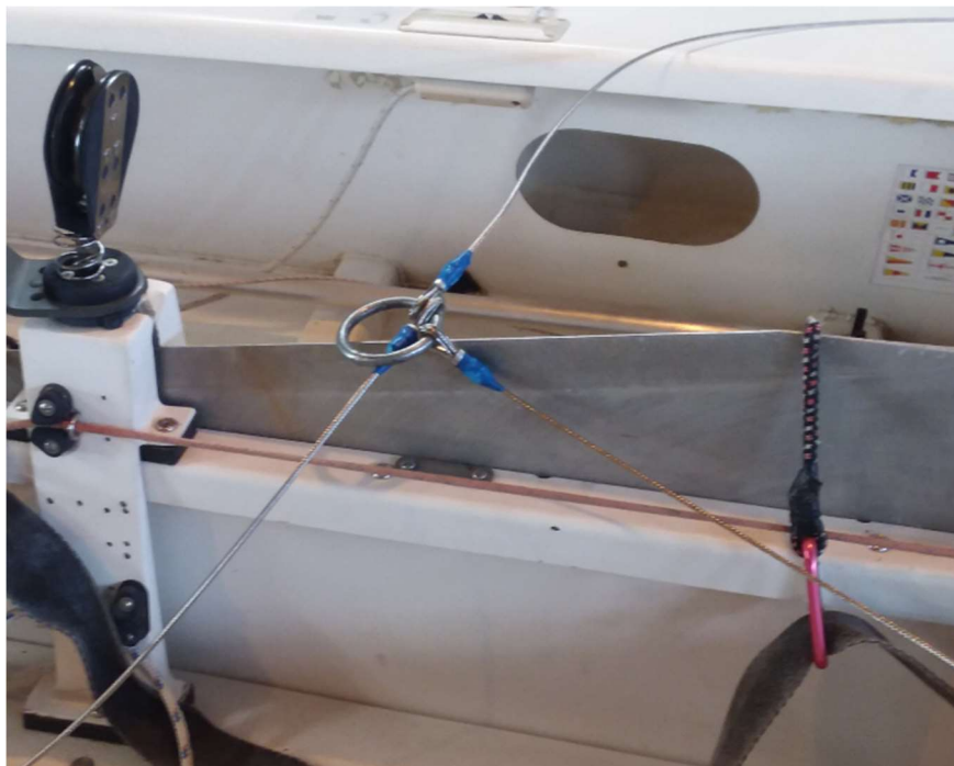
Newly made lifting bridle finished and tested:
