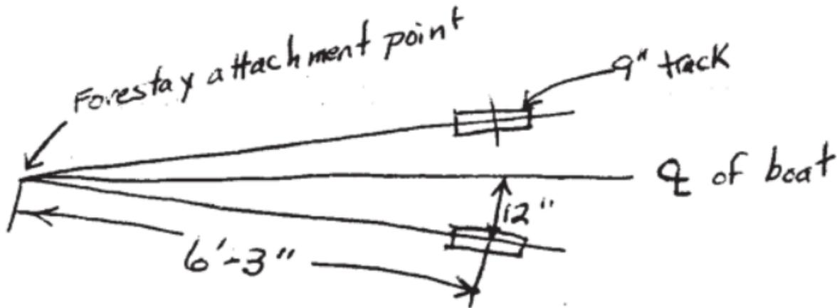
3.15.3 Jib Attachment—The tack of the jib shall be attached to the deck a minimum of 5' 11-1/8" forward of the mast line. And not more than 4 1/2" above the deck.
