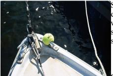
Spinnaker lines seem to seek out the open jaws of the bow chocks to entangle themselves. Closing the chock opening with duct tape works well but a tennis ball is a reusable resource. Cut a hole on two opposite sides of a tennis ball, stuff it in the opening, and do away with snagged spinnaker lines.
