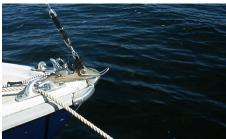
Do you want to catch and stop the spinnaker sheets from going under your Ensign? You can fashion a small wire bowsprit from a heavy coat hanger, or a six inch pegboard loop will work just fine. It can be attached to the bow stem plate with duct tape or black electrical tape. No more running over the lines.
