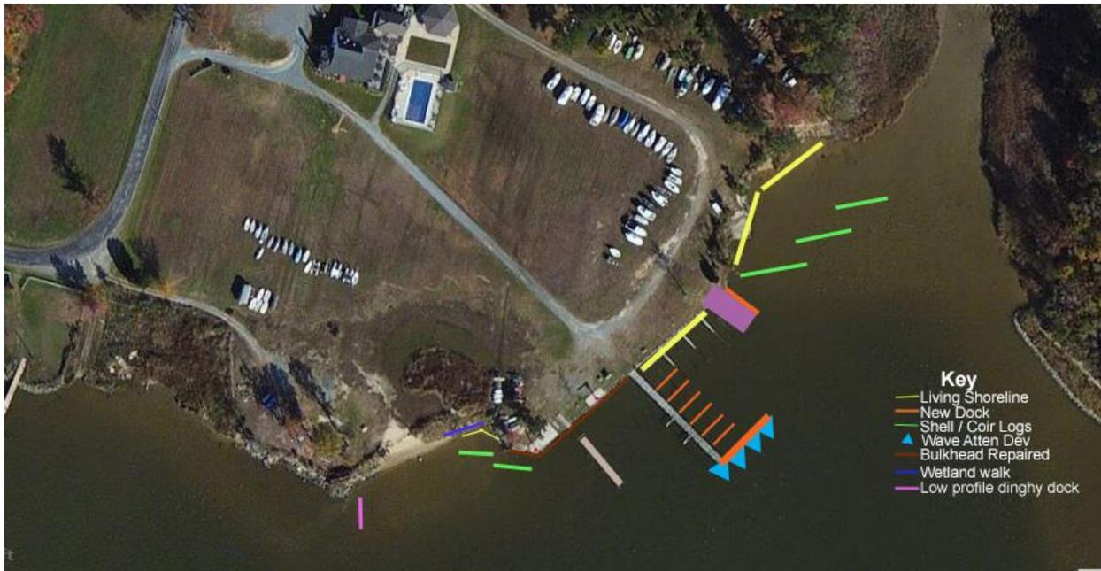
Figure 13. RHYC Waterfront Stabilization Concept
