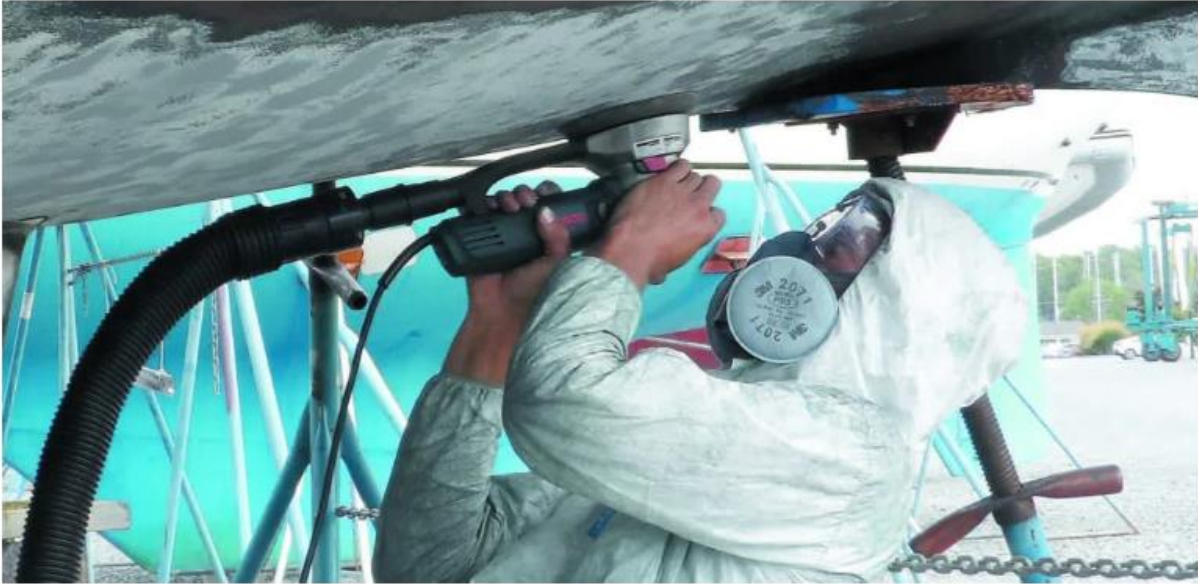
When sanding bottom paint, use only NIOSH-rated high efficiency filters (see "The Best Respirators for the Boatyard". Practical Sailor September September 2017). Do not use disposable fabric masks – they do not provide the same level of protection. Goggles and a hood further increases protection, but they can be hard to bear if it is hot.
